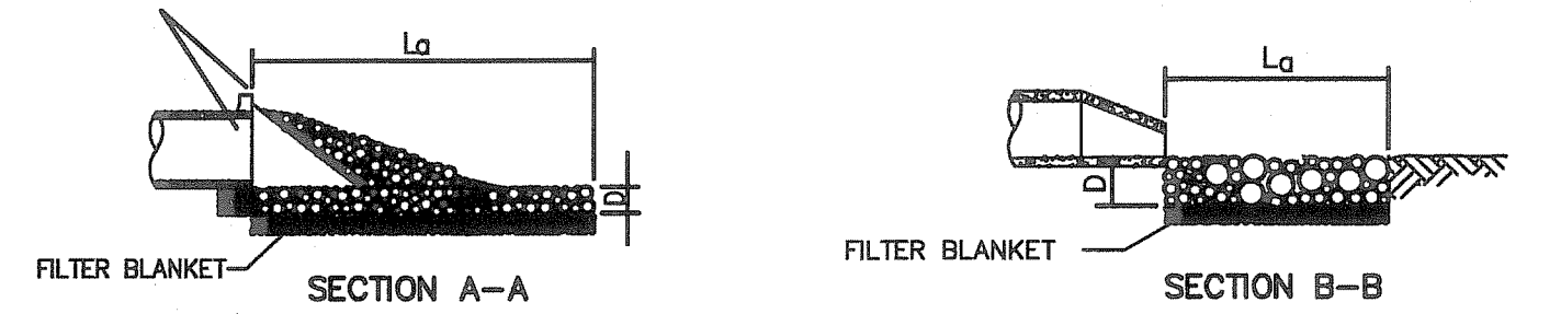
PIPE OUTLET TO WELL-DEFINED CHANNEL: PIPE OUTLET TO FLAT AREA - NO WELL-DEFINED CHANNEL:
