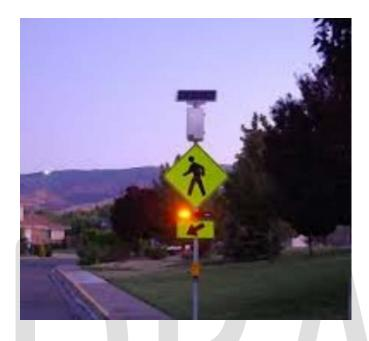
Flashing Sign Beacon – A yellow beacon used to highlight a warning sign or stop sign.
