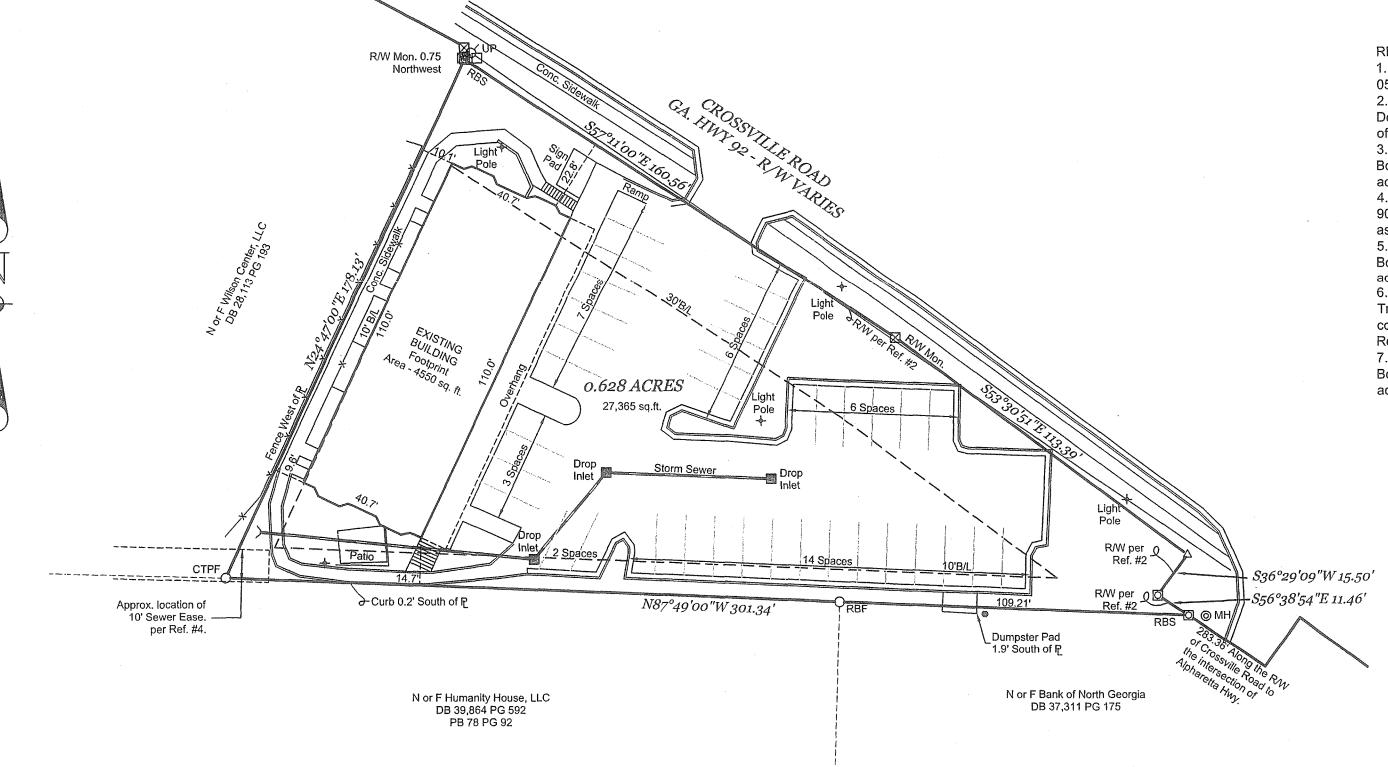
LEGEND Open Top Pin Found Crimp Top Pin Found CTPF CTPS RBF RBS Crimp Top Pin Set Rebar Found Rebar Set B/L Building Line Utility Pole Now or Formerly N or F Fence Overhead Wire Not to Scale Calculated Point
